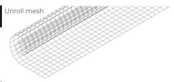
Use a cable ties to hold the edges of the mesh to the 5. wire frame all the way around the balcony
