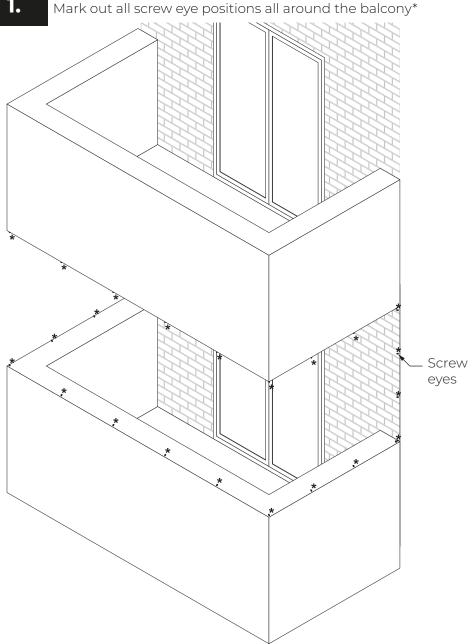
Fix screw eyes to the wall/floor/ceiling with rawl plugs
