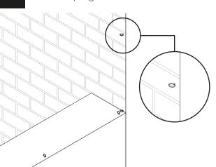
Thread the wire through all of the screw eyes. Tie each open end to the wire tensioner.
